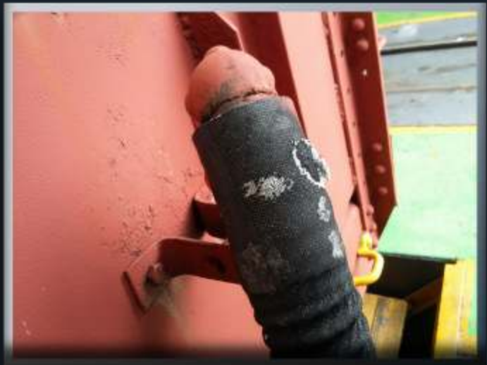
Below left: 2 DZ wagons on the Inspection pit. Below right: Vacuum hose due for retirement.
