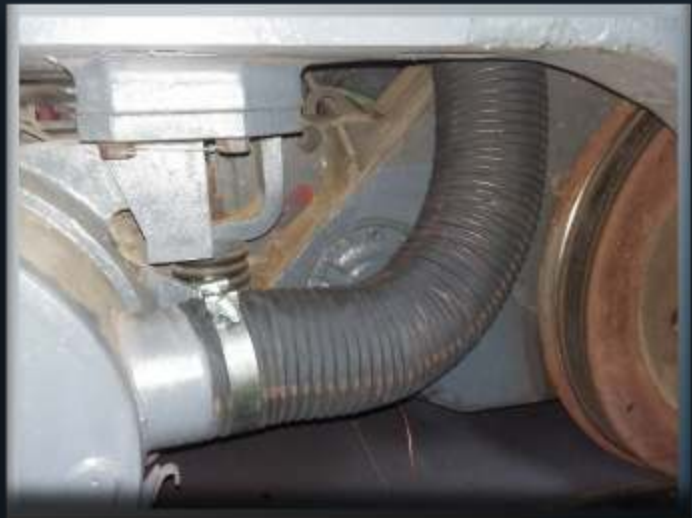
Below left: Thinus cleaning the radiator from above. Below right: The air vent pipe fitted to one of the traction motors.
