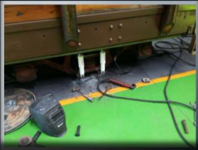
Below: A short test run with the shock absorbers fitted
