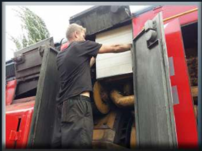
Below: Air filters being changed.
