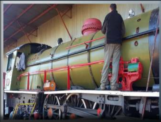
Below: Wouter busy fitting back the hand rails that were removed to fit the cladding.
