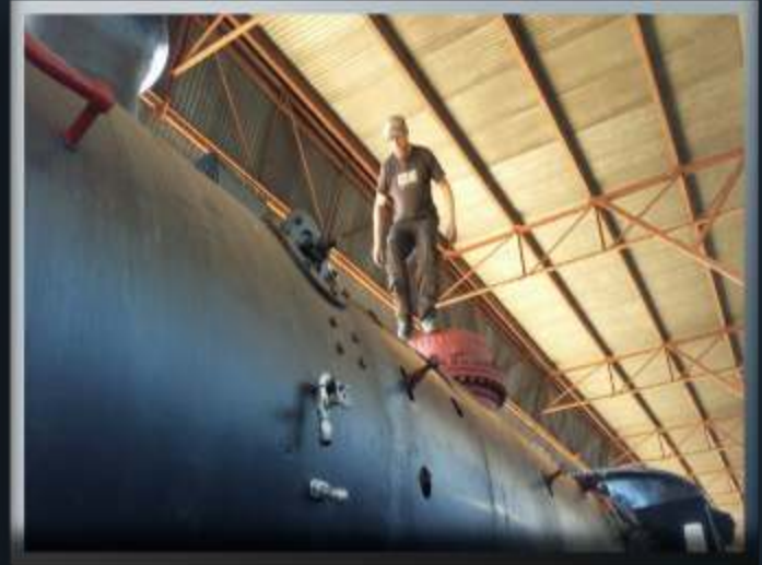
Below: Wouter busy fitting back the hand rails that were removed to fit the cladding.
