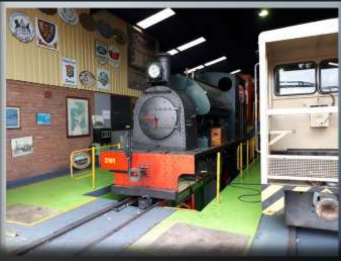
Last week we shunted the Peckett to the inspection pit for under frame inspection as well as for valve setting. the valves were set and we tested her last Friday.
