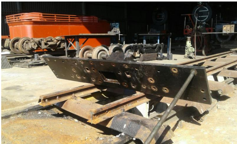
The buffer beam after being re-aligned.
