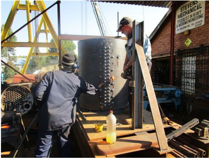
Riveting up butt strap
