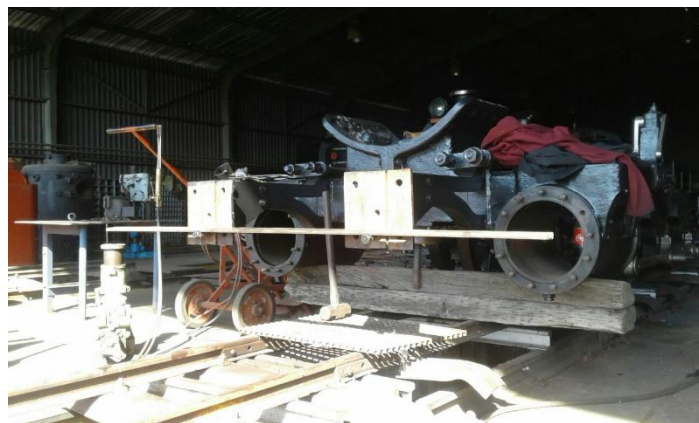
Setting up the alignment of the buffer beam.
