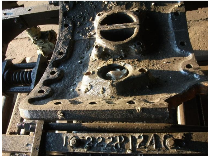
The NG10 boiler saddle casting.
