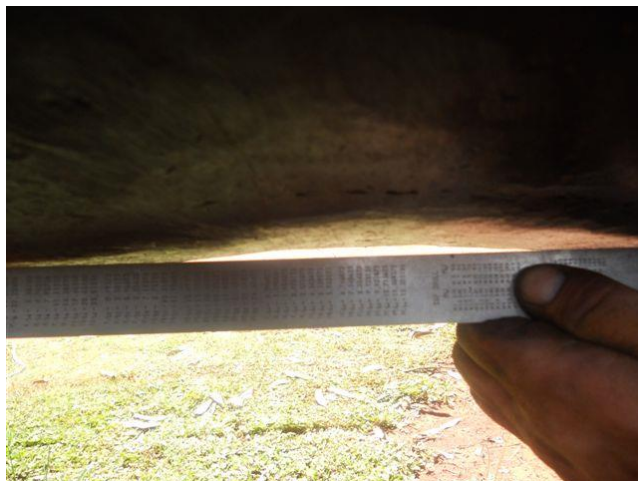
The extent of the bulge in the NG10 boiler barrel
