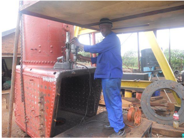
The throat plate stays being drilled out
