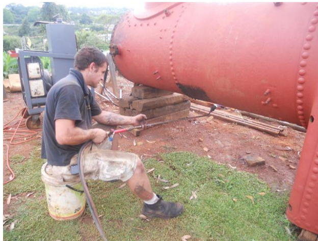
The extent of the bulge in the NG10 boiler barrel
