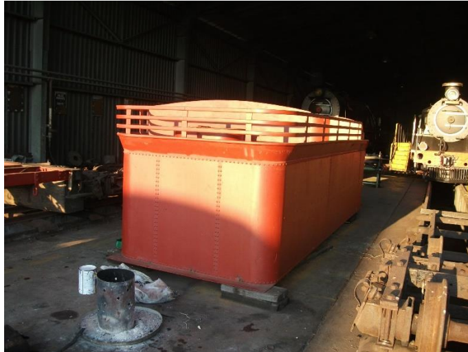
The new tender tank.
