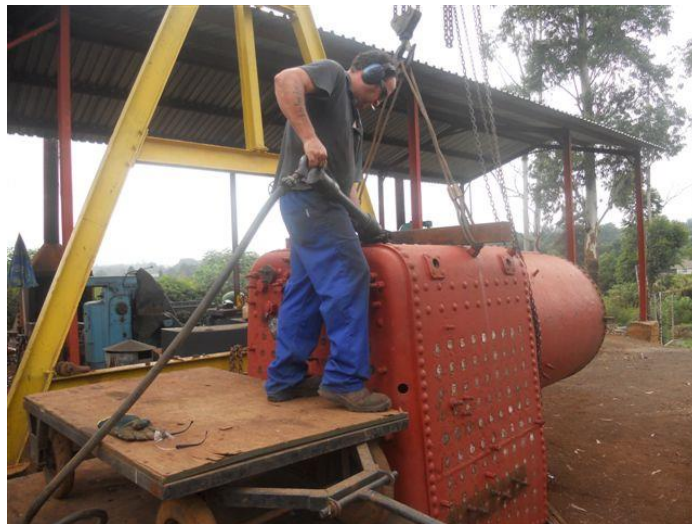
Cutting the stay heads off
