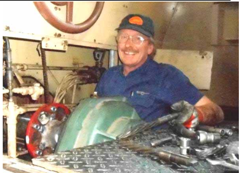
Above Simon Meade in the bowls of the Bagnall loco reaming the bolt holes of the repaired drive shaft coupling . Simon is a loco driver from Bennetsbrook railway near Perth .
