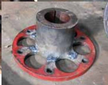
Left After a battle to get the flange off the final drive gearbox it was welded in the main farm workshop overnight .
