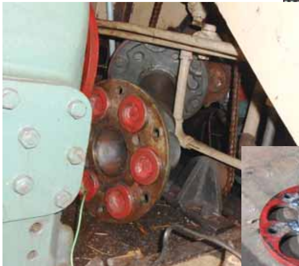
Below . The drive shaft probably broke as a result of the loco being shunted with the gearbox end disconnected
